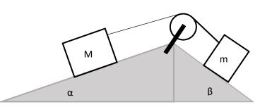
Calculate the tension in the string and the acceleration of the blocks.
