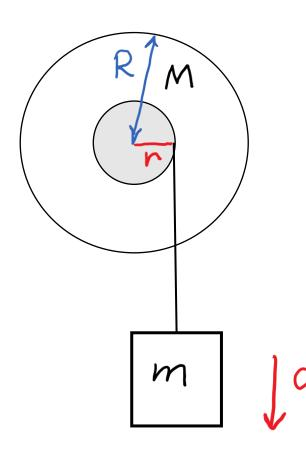
A small disk of radius r is glued onto a large disk of radius R that is mounted on a fixed axle through its center. The combined moment of inertia of the disks is I. A string is wrapped around the edge of the small disk, and a box of mass m is tied to the end of the string. The string does not slip on the disk.
