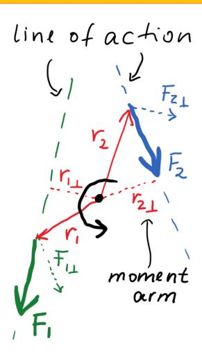
$$\tau_{1z} = +F_1 r_{1\perp} = +F_{1\perp} r_1$$
