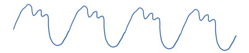
We will only study sine-shaped waves, because all periodic functions can be expressed as a superposition of different sine functions.
