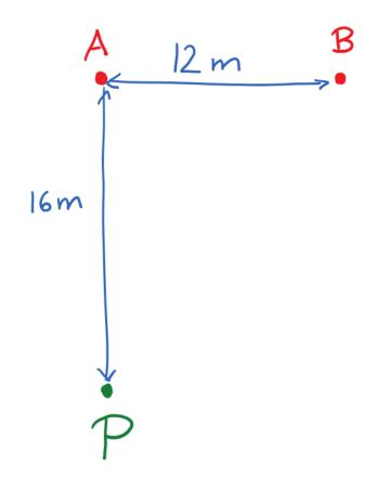
Two loudspeakers emit waves of frequency 172 Hz. The speed of sound is 344 m/s. You are 8 m from speaker A. How close can you get to speaker B and have destructive interference?
