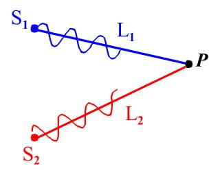
Two sources, waves emitted in phase. How do waves combine at P?
