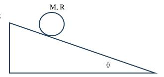
b) (40 points) (OSE) Use force and torque methods to derive the disk's linear acceleration.
